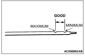
6. Stop the engine and check to ensure that the engine oil level is within the level range indicated on the dip stick.
