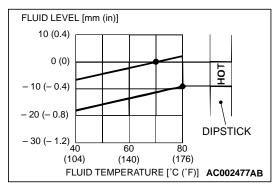
NOTE: If it takes some amount of time until the A/T fluid reaches its normal operating temperature [70 – 80°C (158 – 176°F)], check the A/T fluid level by referring to the left diagram.
