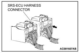
Since the SRS-ECU harness connector is plated to improve conductivity, observe the warning below when checking this connector.
