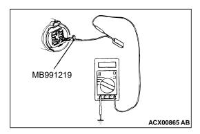
From back side of the connector (SRS-ECU harness side connector)
