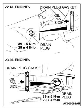
3. Replace the drain plug gasket with a new one, and then tighten the drain plug to the specified torque.
