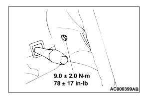
2. Tighten the air bag module mounting screws to 9.0  $\pm$  2.0 N·m (78  $\pm$  17 in-lb).
