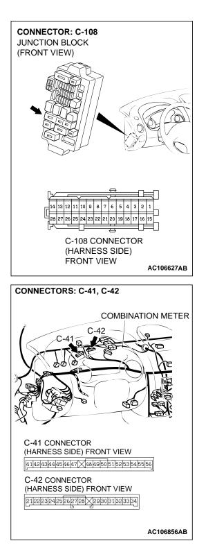
STEP 7. Check the harness for short circuit to ground between junction block connector C-108 (terminal No.25) and combination meter connector C-41 (terminal No.52). NOTE: After inspecting intermediate connectors C-42, inspect the wiring harness. If intermediate connectors are damaged, repair or replace them. Refer to GROUP 00E, Harness Connector Inspection P.00E-2. Then go to Step 10.
