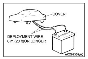
5. Connect the side-airbag module two-pin connector to special tool MB686560 and move the deployment wires out of the vehicle.
