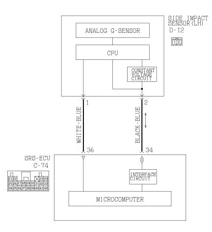
Side Impact Sensor (LH) Power Supply Circuit
