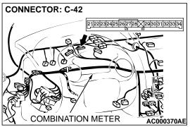
STEP 3. Check the harness for short circuit to ground between SRS-ECU connector C-72 (terminal No.3) and combination meter connector C-42 (terminal No.25). Q: Is the harness wire between the SRS-ECU connector C-
