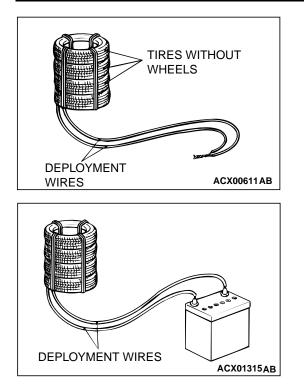
6. Place three old tires without wheels on top of the tire secured to the air bag module, and secure all tires together with ropes (four locations).
