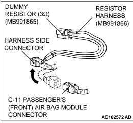
(2) Connect special tool MB991865 to special tool MB991866.
