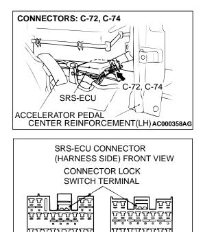
STEP 2. Check SRS-ECU connector C-72 <Vehicles without SRS side air bag>/C-72 and C-74 <Vehicles with SRS side air bag> for damage. If SRS-ECU connectors C-72 and C-74 are damaged, repair or replace them.
