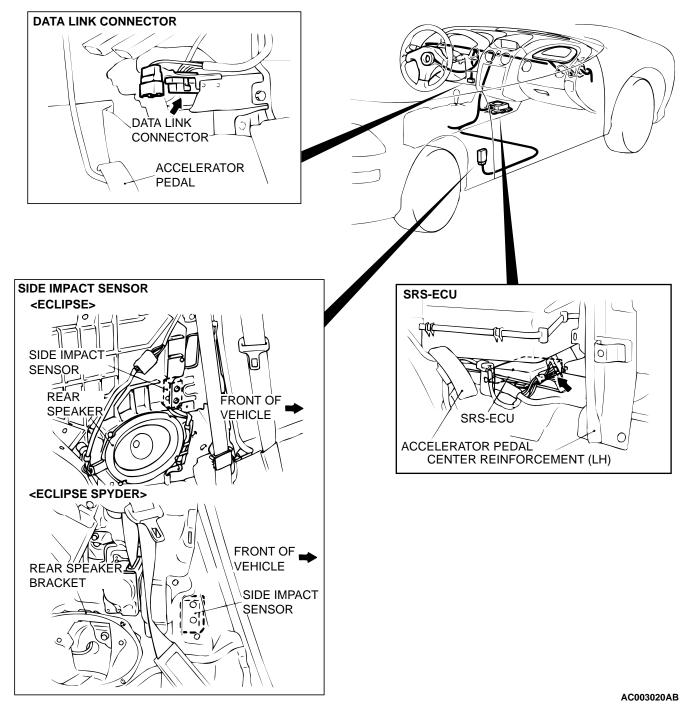
NOTE: The illustration above shows the side impact sensor (LH). The position of the side impact sensor (RH) is symmetrical to this.
