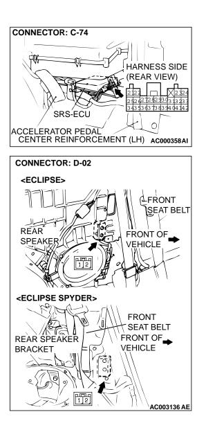
STEP 2. Check the harness wires between SRS-ECU connector C-74 (terminal No.40 and 42) and side impact sensor (RH) connector D-02 (terminal No.1 and 2).
