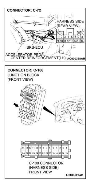
STEP 9. Check the harness for short circuit ground between SRS-ECU connector C-72 (terminal No.24) and junction block connector C-108 (terminal No.12).
