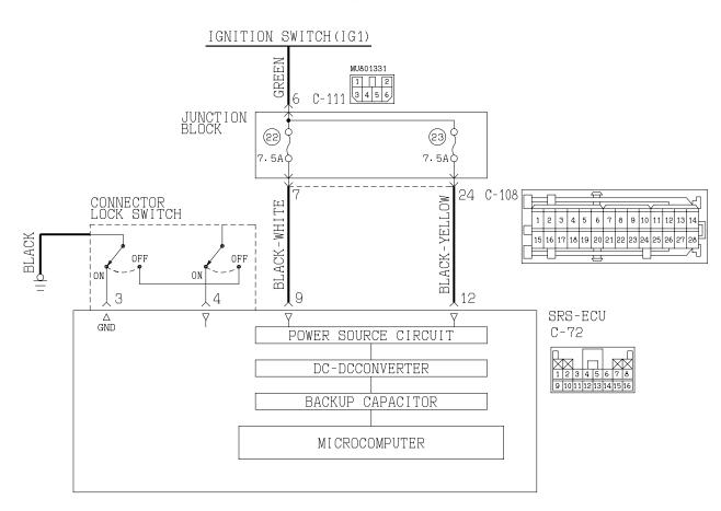
IG1 Power Circuit System (Fuse No.22 Circuit)
