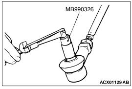
Move the ball joint stud several times and install the nut on the stud. Measure the ball joint breakaway torque with special tool MB990326.
