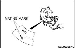
Turn the spring off approximately three turns counterclockwise to align the mating marks.
