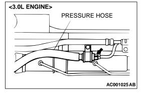
2. Install the pressure hose at the power steering oil pump side as shown in the illustration.
