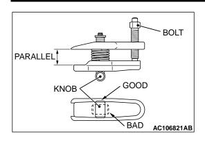
2. After turning the bolt and knob to adjust the insert arms of the special tool MB991897 in parallel, tighten the bolt by hand and confirm that the insert arms are parallel.
