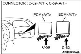
STEP 10. Check for harness damage between right bank heated oxygen sensor (front) connector B-27 terminal 4 and ECM connector C-62 terminal 72 < M/T> or PCM connector C-59 terminal 72 < A/T>.
