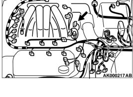
STEP 16. Check for harness damage between camshaft position sensor connector B-22 terminal 5 and ECM connector C-58 terminal 50 <M/T> or PCM connector C-55 terminal 56 <A/T>.
