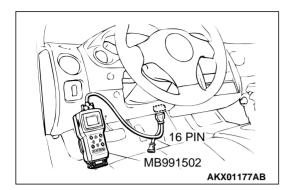
STEP 13. Using scan tool MB991502, check data list item 14: Throttle Position Sensor.
