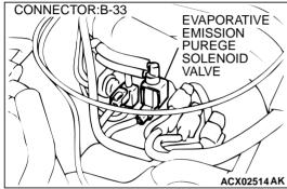
STEP 10. Check for harness damage between MFI relay connector A-21X terminal 1 and evaporative emission purge solenoid connector B-33 terminal 2.
