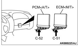
STEP 8. Check connector C-51 at ECM <M/T> or connector C-52 at PCM <A/T> for damage.
