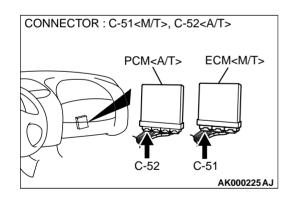
STEP 4. Check connector C-51 at ECM <M/T> or connector C-52 at PCM <A/T> for damage.
