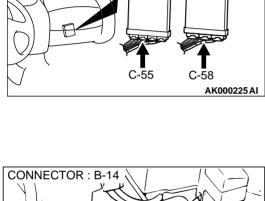
STEP 15. Check connector B-14 at barometric pressure sensor for damage.
