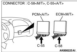
STEP 10. Check for harness damage between generator connector B-45 terminal 4 and ECM connector C-58 terminal 52 <M/T> or PCM connector C-55 terminal 54 <A/T>
