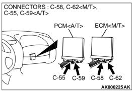
A voltage proportional to the pressure in the intake manifold plenum is sent from the manifold differential pressure sensor output terminal (terminal 1) to the ECM (terminal 92) <M/T> or PCM (terminal 91) <A/T>.
