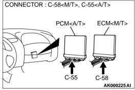
STEP 4. Check connector B-14 at the barometric pressure sensor and connector C-58 at ECM <M/T> or connector C-55 at PCM <A/T> for damage.
