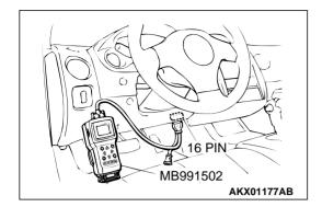
STEP 5. Using scan tool MB991502, check data list item 39: Heated Oxygen Sensor Bank 1, Sensor 1 (right front).
