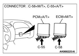
A voltage that is proportional to the atmospheric pressure is sent to the ECM (terminal 51) <M/T> or PCM (terminal 55) <A/T> from the barometric pressure sensor output terminal (terminal 2).
