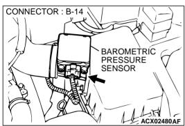
CONNECTOR: C-58<M/T>, C-55<A/T> ECM<M/T> PCM<A/T> C-55 AK000225 AI STEP 13. Check connector B-14 at the barometric pressure sensor and connector C-58 at ECM <M/T> or connector C-55 at PCM <A/T> for damage.
