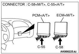
STEP 10. Check for short circuit to ground between crankshaft position sensor connector B-20 terminal 2 and ECM connector C-58 terminal 43 <M/T> or PCM connector C-55 terminal 45 <A/T>.
