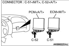
STEP 7. Check for open circuit or short circuit to ground between left bank heated oxygen sensor (front) connector B-24 terminal 3 and ECM connector C-51 terminal 3 < M/T > or PCM connector C-52 terminal 3 <A/T>.
