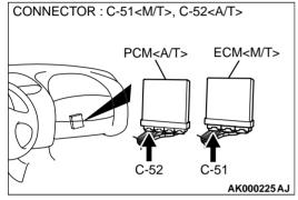
STEP 8. Check for open circuit and short circuit to ground between evaporative emission purge solenoid connector B-33 terminal 1 and ECM connector C-51 terminal 16 < M/T > or PCM connector C-52 terminal 34 < A/T >.
