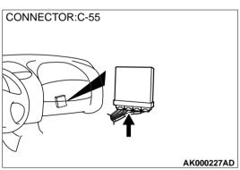
STEP 5. Check for open circuit and short circuit to ground and harness damage between park/neutral position switch connector B-41 terminal 9 and PCM connector C-55 terminal 58.
