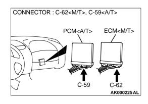
STEP 9. Check connector C-62 at ECM <M/T> or connector C-59 at PCM <A/T> for damage.
