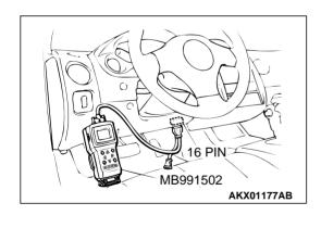
STEP 14. Using scan tool MB991502, check data list item 27: Power Steering Pressure Switch.
