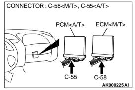
STEP 5. Check for open circuit between engine coolant temperature sensor connector B-11 terminal 1 and ECM connector C-58 terminal 44 <M/T> or PCM connector C-55 terminal 44 <A/T>.
