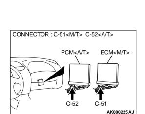
STEP 8. Check connector C-51 at ECM <M/T> or connector C-52 at PCM <A/T> for damage.
