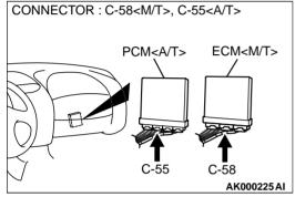
STEP 17. Check for harness damage between intake air temperature sensor connector B-14 terminal 5 and ECM connector C-58 terminal 49 <M/T> or PCM connector C-55 terminal 57 <A/T>.
