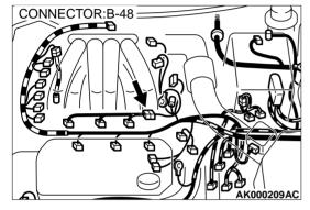
STEP 8. Check connector B-01, B-02, B-05, B-06, B-25, B-26 at injector and connector B-118 at injector intermediate connector for damage.
