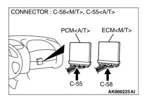
STEP 4. Check connector C-58 at ECM <M/T> or connector C-55 at PCM <A/T> for damage.
