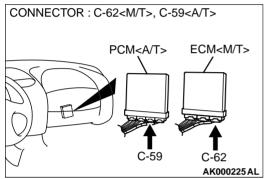
STEP 13. Check for short circuit to ground and harness damage between left bank heated oxygen sensor (rear) connector B-23 terminal 4 and ECM connector C-62 terminal 73 <M/T> or PCM connector C-59 terminal 73 <A/T>.
