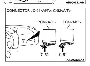
STEP 10. Check for harness damage between left bank heated oxygen sensor (front) connector B-24 terminal 3 and ECM connector C-51 terminal 3 <M/T> or PCM connector C-52 terminal 3 <A/T>.
