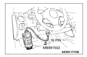
STEP 1. Using scan tool MB991502, read the A/T diagnostic trouble code (DTC).
