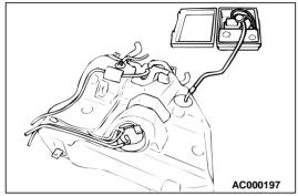
(2) Connect an evaporative emission system pressure pump to the leveling valve nipple.
