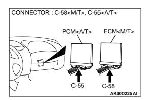
STEP 10. Check connector C-58 at ECM <M/T> or connector C-55 at PCM <A/T> for damage.
