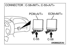
STEP 7. Check connector C-58 at ECM <M/T> or connector C-55 at PCM <A/T> for damage.
