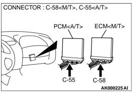
STEP 8. Check for open circuit and harness damage between manifold differential pressure sensor connector B-04 terminal 2 and ECM connector C-58 terminal 49 < M/T > or PCM connector C-55 terminal 57 < A/T >.
