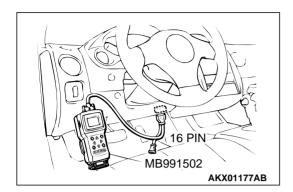
STEP 1. Using scan tool MB991502, check data list item 12: Volume Air Flow Sensor.
