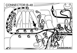
STEP 5. Check connector B-48 at injector intermediate connector for damage.
