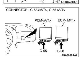
STEP 11. Check for short circuit to ground between barometric pressure sensor connector B-14 terminal 1 and ECM connector C-58 terminal 42 <M/T> or PCM connector C-55 terminal 46 <A/T>.
