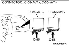
STEP 14. Check for open circuit and harness damage between intake air temperature sensor connector B-14 terminal 5 and ECM connector C-58 terminal 49 <M/T> or PCM connector C-55 terminal 57 <A/T>.
