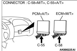
STEP 10. Check for harness damage between manifold differential pressure sensor connector B-04 terminal 3 and ECM connector C-58 terminal 42 < M/T> or PCM connector C-55 terminal 46 < A/T>.
