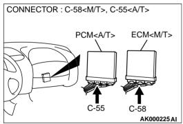
STEP 8. Check for open circuit and short circuit to ground between generator connector B-45 terminal 4 and ECM connector C-58 terminal 52 <M/T> or PCM connector C-55 terminal 54 <A/T>.
