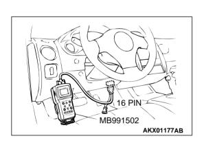
STEP 5. Using scan tool MB991502, check data list item 25: Barometric Pressure Sensor.
