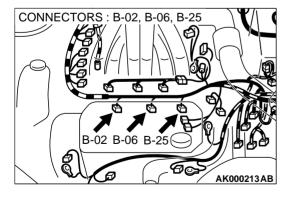
STEP 5. Check connector B-02, B-06, B-25 at left bank injector for damage.
