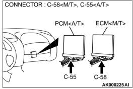
STEP 9. Check for open circuit between barometric pressure sensor connector B-14 terminal 5 and ECM connector C-58 terminal 49 <M/T> or PCM connector C-55 terminal 57 <A/T>.
