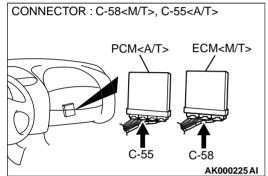
STEP 13. Check for harness damage between engine coolant temperature sensor connector B-11 terminal 1 and ECM connector C-58 terminal 44 < M/T> or PCM connector C-55 terminal 44 < A/T>.
