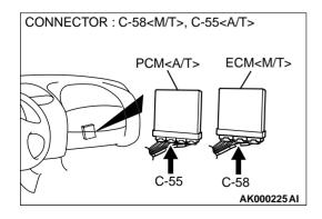
STEP 12. Check connector C-58 at ECM <M/T> or connector C-55 at PCM <A/T> for damage. Q: Is the connector in good condition?
