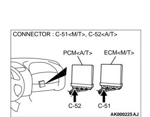
STEP 9. Check connector C-51 at ECM <M/T> or connector C-52 at PCM <A/T> for damage.
