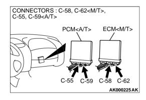
STEP 10. Check connector C-58, C-62 at ECM <M/T> or connector C-55, C-59 at PCM <A/T> for damage.
