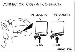
STEP 18. Check for harness damage between intake air temperature sensor connector B-14 terminal 6 and ECM connector C-58 terminal 62 <M/T> or PCM connector C-55 terminal 64 <A/T>.
