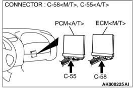
STEP 10. Check for open circuit and harness damage between left bank heated oxygen sensor (rear) connector B-23 terminal 2 and ECM connector C-58 terminal 49 < M/T > or PCM connector C-55 terminal 57 < A/T >.
