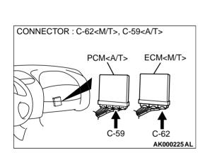
STEP 11. Check connector C-62 at ECM <M/T> or connector C-59 at PCM <A/T> for damage.
