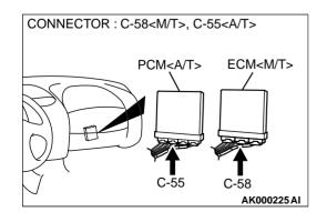
STEP 12. Check connector C-58 at ECM <M/T> or connector C-55 at PCM <A/T> for damage.
