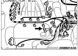
STEP 10. Check for harness damage between left bank heated oxygen sensor (rear) connector B-23 terminal 3 and ECM connector C-51 terminal 26 <M/T> or PCM connector C-52 terminal 26 <A/T>.
