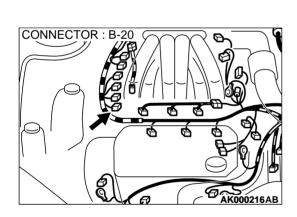
STEP 18. Check for harness damage between crankshaft position sensor connector B-20 terminal 1 and ground. Q: Is the harness wire in good condition?
