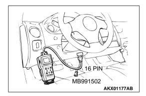
STEP 1. Using scan tool MB991502, check data list item 16: Power Supply Voltage.
