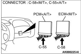
STEP 10. Check for open circuit and harness damage between left bank heated oxygen sensor (front) connector B-24 terminal 2 and ECM connector C-58 terminal 49 < M/T > or PCM connector C-55 terminal 57 <A/T>.
