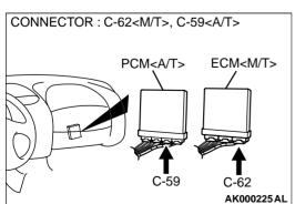
STEP 4. Check connector B-23 at left bank heated oxygen sensor (rear) and connector C-62 at ECM <M/T> or connector C-59 at PCM <A/T> for damage.
