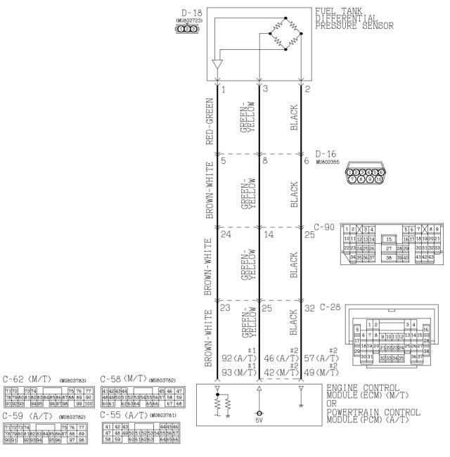
NOTE \*1:ECM connector C-62(M/T)or PCM connec tor C-59(A/T) \*2:ECM connector C-58(M/T)or PCM connec tor C-55(A/T)
