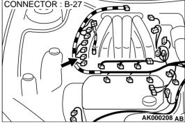
STEP 10. Check for harness damage between right bank heated oxygen sensor (front) connector B-27 terminal 3 and ECM connector C-51 terminal 4 < M/T> or PCM connector C-52 terminal 4 <A/T>.
