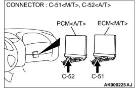
STEP 7. Check for open circuit or short circuit to ground between right bank heated oxygen sensor (front) connector B-27 terminal 3 and ECM connector C-51 terminal 4 <M/T> or PCM connector C-52 terminal 4 <A/T>. Q: Is the harness wire in good condition?
