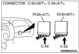
STEP 13. Check for short circuit to ground and harness damage between right bank heated oxygen sensor (rear) connector B-28 terminal 4 and ECM connector C-62 terminal 74 <M/T> or PCM connector C-59 terminal 74 <A/T>
