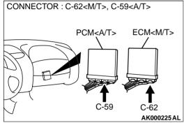
STEP 8. Check for harness damage between left bank heated oxygen sensor (front) connector B-24 terminal 4 and ECM connector C-62 terminal 71 < M/T> or PCM connector C-59 terminal 71 < A/T>.
