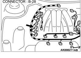
STEP 10. Check for harness damage between right bank heated oxygen sensor (rear) connector B-28 terminal 3 and ECM connector C-51 terminal 27 < M/T > or PCM connector C-52 terminal 27 <A/T>.
