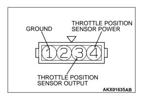
3. Connect an ohmmeter between terminals 1 (ground) and 3 (output), or between terminals 3 (output) and 4 (power). Then, make sure that the resistance changes smoothly when the throttle valve is slowly moved to the fully open position.
