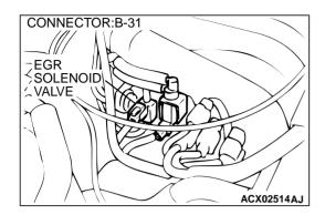
STEP 11. Check for harness damage between EGR solenoid connector B-31 terminal 2 and ECM connector C-51 terminal 6 <M/T> or PCM connector C-52 terminal 6 <A/T>
