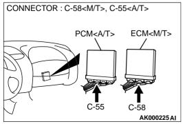
STEP 8. Check for open circuit between distributor connector B-22 terminal 2 and ECM connector C-58 terminal 45 <M/T> or PCM connector C-55 terminal 43 <A/
