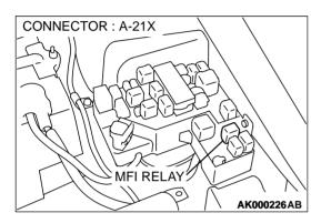
STEP 8. Check for harness damage between MFI relay connector A-21X terminal 1 and injector intermediate connector B-48 terminal 1.
