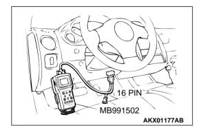
STEP 1. Using scan tool MB991502, check actuator test item 08: Evaporative Emission Purge Solenoid.
