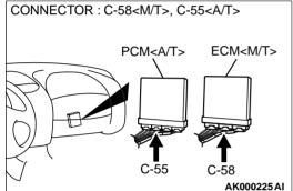
STEP 10. Check for open circuit and harness damage between right bank heated oxygen sensor (rear) connector B-28 terminal 2 and ECM connector C-58 terminal 49 < M/T > or PCM connector C-55 terminal 57 <A/T>.
