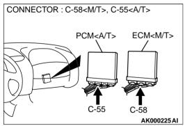
STEP 5. Check for open circuit and short circuit to ground between manifold differential pressure sensor connector B-04 terminal 3 and ECM connector C-58 terminal 42 < M/T > or PCM connector C-55 terminal 46 < A/T >.
