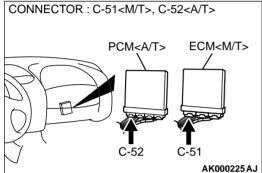
STEP 3. Check for open circuit and short circuit to ground and harness damage between fan controller A-30 terminal 2 and ECM connector C-51 terminal 18 < M/T > or PCM connector C-52 terminal 18 < A/T >.
