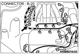
STEP 16. Check for harness damage between MFI relay connector A-21X terminal 1 and crankshaft position sensor connector B-20 terminal 3.
