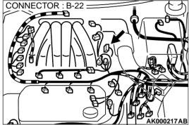
STEP 15. Check for harness damage between MFI relay connector A-21X terminal 1 and camshaft position sensor connector B-22 terminal 6.
