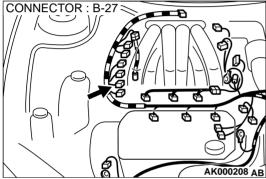
STEP 9. Check for harness damage between MFI relay connector A-21X terminal 1 and right bank heated oxygen sensor (front) connector B-27 terminal 1.
