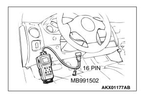
STEP 10. Using scan tool MB991502, check data list item 14: Throttle Position Sensor.
