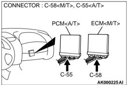
STEP 12. Check for harness damage between left bank heated oxygen sensor (rear) connector B-23 terminal 2 and ECM connector C-58 terminal 49 <M/T> or PCM connector C-55 terminal 57 <A/T>.
