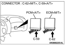
STEP 4. Check for open circuit, short circuit to ground and harness damage between knock sensor connector B-35 terminal 1 and ECM connector C-62 terminal 91 <M/T> or PCM connector C-59 terminal 90 <A/T>.
