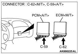
STEP 7. Check for harness damage between throttle position sensor connector B-07 terminal 3 and ECM connector C-62 terminal 78 < M/T> or PCM connector C-59 terminal 78 < A/T>.
