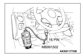
STEP 8. Using scan tool MB991502, check data list item 14: Throttle Position Sensor.
