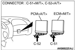
STEP 5. Check for open circuit and short circuit to ground and harness damage between generator connector B-45 terminal 1 and ECM connector C-51 terminal 8 < M/T> or PCM connector C-52 terminal 8 < A/T>.
