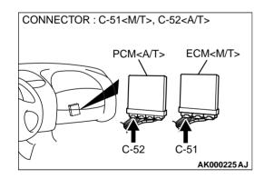
STEP 9. Check connector C-51 at ECM <M/T> or connector C-52 at PCM <A/T> for damage.
