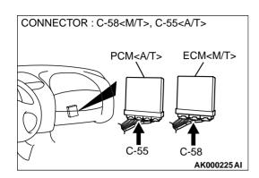
STEP 7. Check connector C-58 at ECM <M/T> or connector C-55 at PCM <A/T> for damage.
