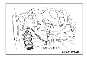
STEP 1. Using scan tool MB991502, check data list item 39: Heated Oxygen Sensor Bank 1, Sensor 1 (right front).
