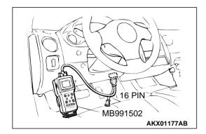
STEP 1. Using scan tool MB991502, check actuator test item 02, 04, 06: Injectors.
