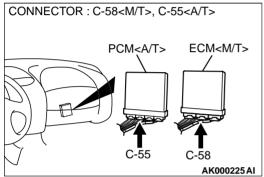
STEP 10. Check for harness damage between engine coolant temperature sensor connector B-11 terminal 2 and ECM connector C-58 terminal 49 < M/T> or PCM connector C-55 terminal 57 < A/T>.
