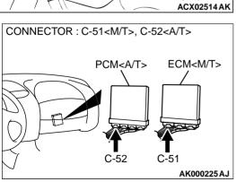
STEP 11. Check for harness damage between evaporative emission purge solenoid connector B-33 terminal 1 and ECM connector C-51 terminal 16 < M/T > or PCM connector C-52 terminal 34 <A/T>.
