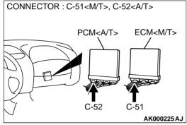
STEP 3. Check connector B-14 at volume air flow sensor and connector C-51 at ECM <M/T> or connector C-52 at PCM <A/T> for damage.
