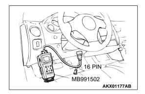
STEP 1. Using scan tool MB991502, check data list item 12: Volume Air Flow Sensor.
