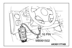
STEP 1. Using scan tool MB991502, check data list item 95: Manifold Differential Pressure Sensor.
