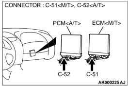
STEP 7. Check for open circuit between distributor connector B-22 terminal 3 and ECM connector C-51 terminal 11 <M/T> or PCM connector C-52 terminal 11 <A/
