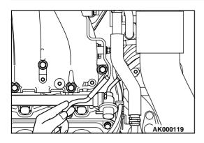
9. Disconnect the vacuum hose (blue stripe) from the fuel pressure regulator and measure fuel pressure with the hose end closed with your finger.
