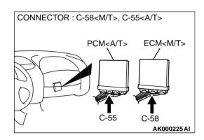
STEP 8. Check connector C-58 at ECM <M/T> or connector C-55 at PCM <A/T> for damage.
