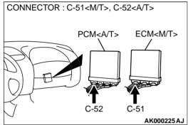
STEP 8. Check for open circuit and short circuit to ground between evaporative emission ventilation solenoid connector D-10 terminal 1 and ECM connector C-51 terminal 35 <M/T> or PCM connector C-52 terminal 35 <A/T>.
