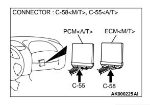
STEP 9. Check connector C-58 at ECM <M/T> or connector C-55 at PCM <A/T> for damage.
