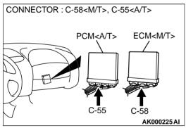
STEP 5. Check for open circuit and short circuit to ground between throttle position sensor connector B-07 terminal 4 and ECM connector C-58 terminal 42 < M/T> or PCM connector C-55 terminal 46 < A/T>.
