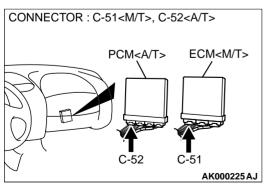
STEP 4. Check for short circuit to ground between volume air flow sensor connector B-14 terminal 7 and ECM connector C-51 terminal 19 <M/T> or PCM connector C-52 terminal 19 <A/T>.
