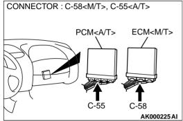
STEP 6. Check for harness damage between throttle position sensor connector B-07 terminal 4 and ECM connector C-58 terminal 42 <M/T> or PCM connector C-55 terminal 46 <A/T>.
