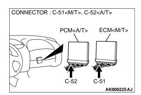
STEP 12. Check the connector C-51 at the ECM <M/T> or connector C-52 at the PCM <A/T> for damage.
