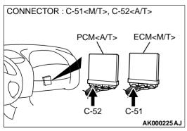
STEP 11. Check for harness damage between evaporative emission ventilation solenoid connector D-10 terminal 1 and ECM connector C-51 terminal 35 < M/T > or PCM connector C-52 terminal 35 < A/T >.
