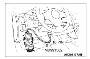
STEP 5. Using scan tool MB991502, check data list item 59: Heated Oxygen Sensor Bank 2, Sensor 2 (left rear).
