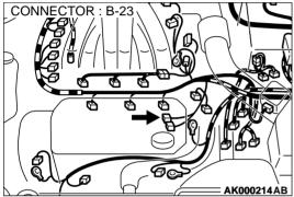
STEP 9. Check for harness damage between MFI relay connector A-21X terminal 1 and left bank heated oxygen sensor (rear) connector B-23 terminal 1.
