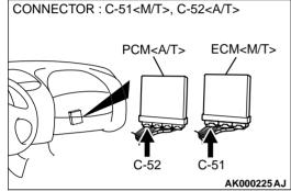
STEP 7. Check for open circuit or short circuit to ground between right bank heated oxygen sensor (rear) connector B-28 terminal 3 and ECM connector C-51 terminal 27 < M/T> or PCM connector C-52 terminal 27 < A/T>.
